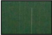
120045 / 125045 LF1 - S2 - O TERRA VERTE PG17 CHROM OXIDE / PW6 TITAN DIOXIDE / PBK11 SYNTH IRON OX / PB29 SOD ALUM SULPHO
