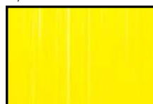
120018 / 125018 LF1 - S1 - 0 CADMIUM YELLOW LIGHT PR35:1 CADMIUM SELENO- SULFIDE COPRECIPATED WITH BARIUM SULFATE
