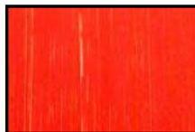
120012 / 125012 LF1 - S4 - 0 CADMIUM RED SCARLET PR108:1 CAD SELENO-SULFIDE COPRECIPATED WITH BARIUM SULFATE
